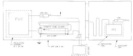
nor appropriate. The EM clamp is often used to test unshielded multiple conductor cables. The figure above shows a typical test setup using the EM Clamp and a ferrite tube decoupling network.
