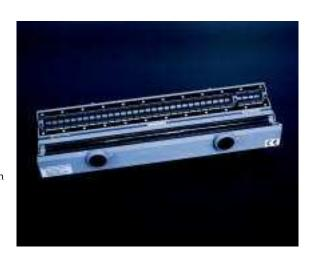
For conducted immunity testing from 150 kHz to 230 MHz the increased efficiency can save the user as much as 100% on required CW amplifier power. The F-203I family requires less than 10 watts to develop the 10 volt open circuit level in accord with IEC 1000-4-6. When an additional ferrite decoupling or ferrite tube is used in the test the F-203I family requires less than 36 watts to develop the 10 volt open circuit level.
